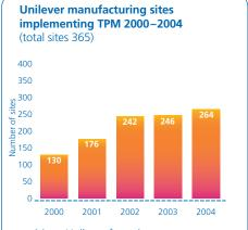
Many Unilever factories use a people-based method of improving efficiency and increasing product quality known as Total Productive Maintenance (TPM). Each employee is involved as a team member, trained to investigate and safely correct any faults, and so eliminate losses.
